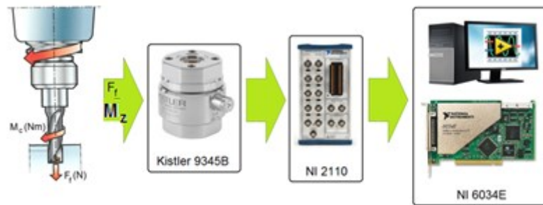
Fig. 4.7. Schematic diagram of the data acquisition system
