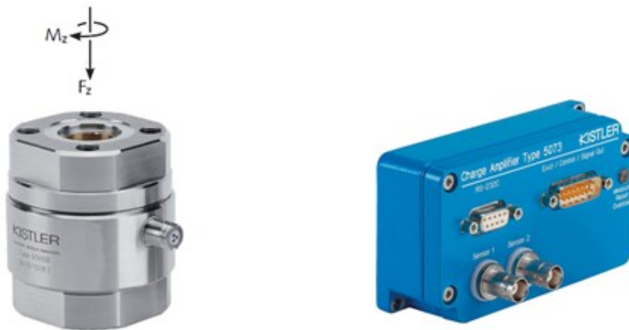
Fig. 4.5. Axial force ( F_z ) and cutting moment ( M_z ) sensor type 9345B2 with 5073A211 charge preamplifier
