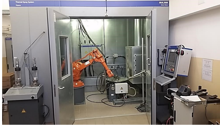
Fig. 2.2. Image of the Sulzer Metco plasma spraying system: the booth with ABB robot
