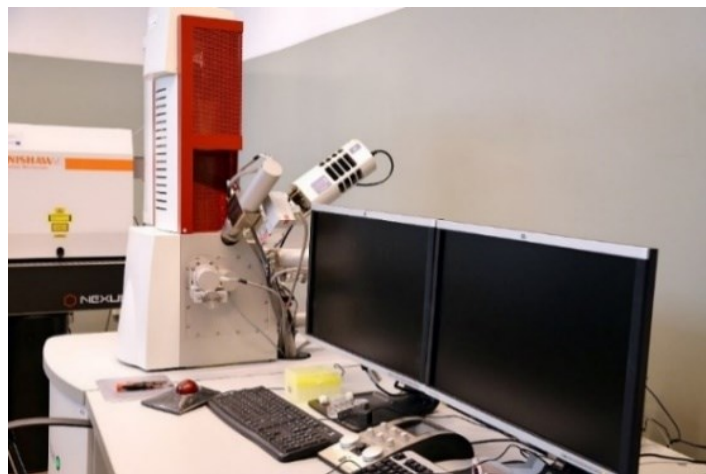
Fig. 4.1. Scanning electron microscope with TESCAN EDS attachment
