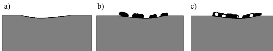
Fig. 2.9. A schematic representation of the mechanism of collision of a metallic powder particle with substrate in conditions as-delivered after thermal spraying: (a) crater; (b) spattering; (c) adhesion with gas blisters
