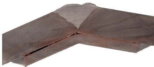
Fig. 1.4. Macrostructure of a welded tee joint of 17-mm thick ArmoX 500T steel plates with backing
