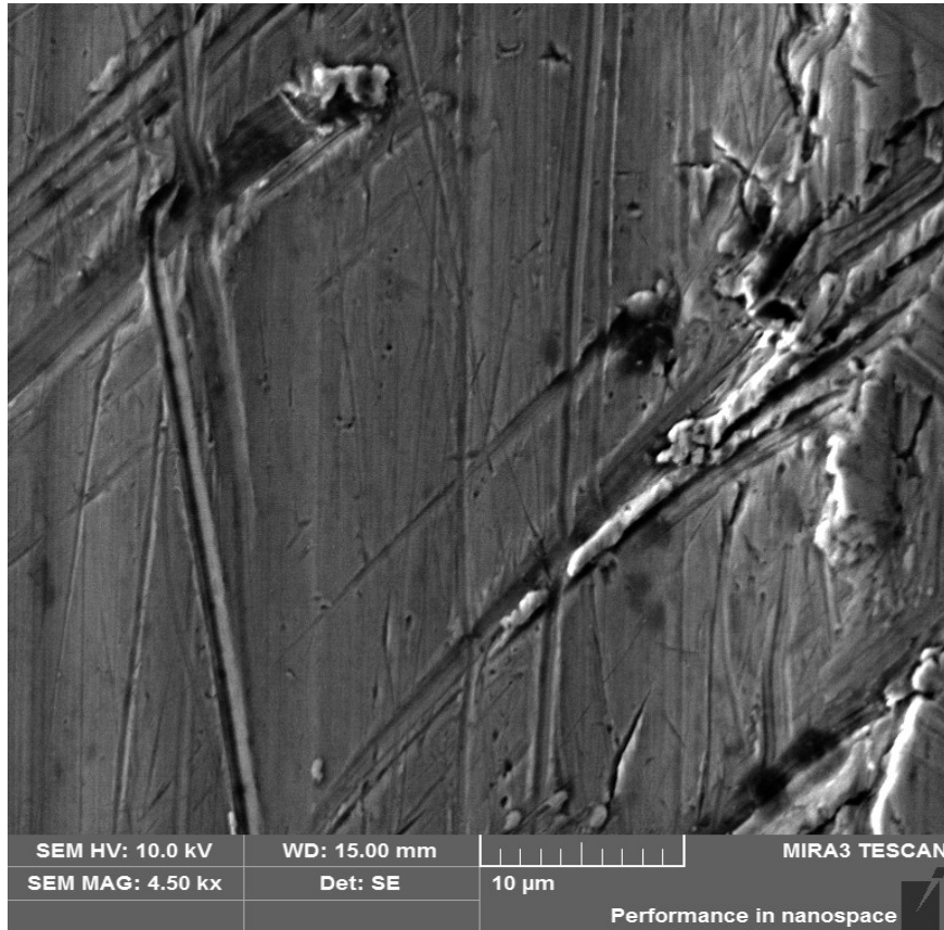
Fig. 4.3. Microphotograph of an Ti6Al4V panel surface
