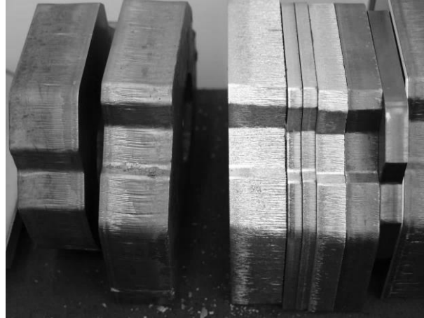
Fig. 1.4. Photographs of laser-cut objects: a) various materials of products, b) elements of considerable thickness [B. Ciecńska]
