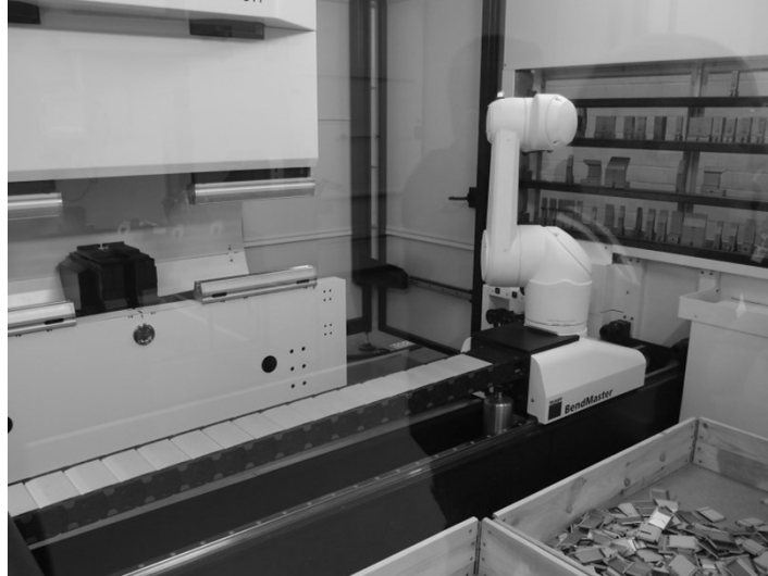
Fig. 1.1. Examples of comprehensive solutions for the Industry 4.0: a) planning and real-time control of the implementation of cutting operations, b) pallets for depositing finished products, c) bending station with a robotic exchanger of fittings [B. Ciecńska]
