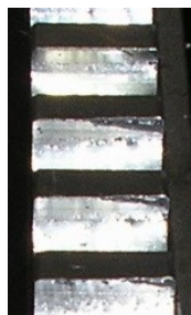
Fig. 2.5. Broach teeth wear during the "dry" cutting.
