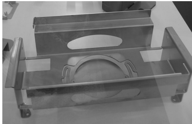
Fig. 1.2. The variety of possibilities of using lasers in the production line: a) cutting various products from one sheet of metal, b) combining cutting and bending of sheet metal in one production socket [B. Ciecńska]
