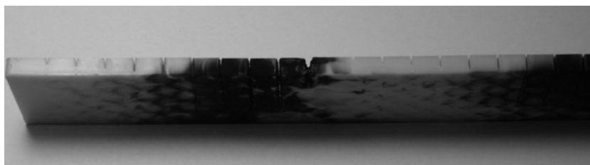
Fig. 1.9. Polypropylene Moplen HP500N laser cutting with talc - side view, composite ignites, gaps on the left side for 150W laser power, on the right side for the power of 113W
